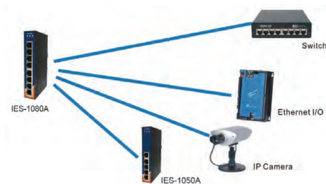
Connections of Ethernet devices
