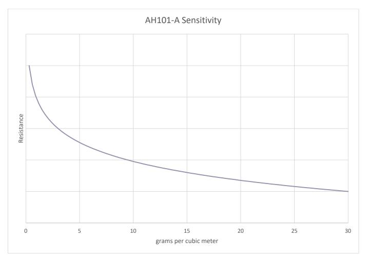
The above transfer function shows the relationship between absolute humidity and the resistance change of the sensing element. As conditions dry out the sensor becomes more sensitive and reactive to moisture.
